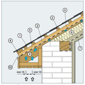
Eaves with soffit ventilation
