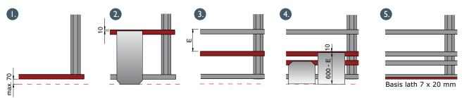
Install the bottom edge of slate in level with eave. The top edge of slate locates the supplementary batten from which we measure all other battens pacing "E"set by roof slope.
