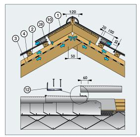
$\label{eq:Ridge} \mbox{Ridge ventilation incorporating slated ridge with fibrecement ridge cupping}$
