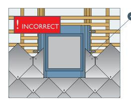
It is possible to fasten this part of slate by only one nail, which is not sufficient.
