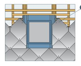
To fasten the slates at edging it is necessary to use an increased number of battens.
