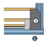
The second cut slate is fastened with two nails. Rivet is pushed under the edge of this cut slate.
