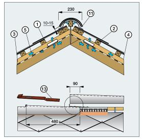
Ridge ventilation incorporating fibrecement ridge capping
