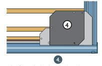
The first whole slate laid so the rivet protrudes through the rivet hole. Rivet for next course of slates is pushed under the edge
