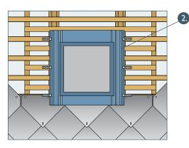
Installation of roof exit on prepared hole, its fastening by clip. Bottom part of window covers the first row of slates.
