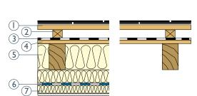
It is possible to use this solution when refurbishing boarded roofs. It is applicable for low pitched of roofs.
