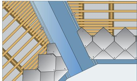
It is not possible to sufficiently fasten marked cut. In winter the ice can lean on this part which can result in breakage.
