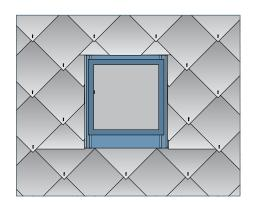
To install Cembrit Quadra we concentrate battens at roof perimeter roof corner, valley, chimney and all penetrations. The following description of installation shows that this preparation is important providing support for smaller cut slates at the edging of penetration holes.
