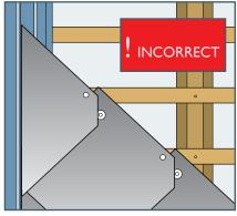
The picture on the right shows a cut slate which is impossible to sufficiently fasten, therefore the slate cut to be as larger layer as a half of slate. All slates must be installed with 3 fixings.
